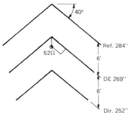
Fig. 2- By tilting the elements forward, gain as well as front-to-back and front-to-side ratios increased. Horizontal beam width decreased.
